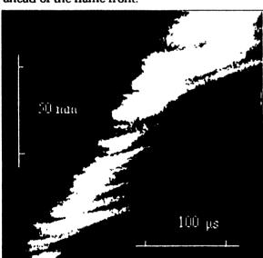
Figure 4. An example of streak photo record of LVD at the front velocity ~ 0 8 km/s with tracks of burning grains [23]. Single-based powder of 3.3 mm effective grain diameter in a multi-section DDT steel tube 15 mm i.d and 700 mm long with a slit for photography at a distance 280 – 420 mm from igniter. Shape of the tracks with an initial horizontal leg of ~ 30 µs long gives evidence that grains ignited with no contribution of a compaction process.
