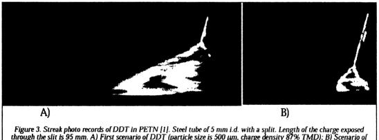
Figure 3. Streak photo records of DDT in PETN [1]. Steel tube of 5 mm i.d. with a split. Length of the charge exposed through the slit is 95 mm. A) First scenario of DDT (particle size is 500 µm, charge density 87% TMD); B) Scenario of DDT with a secondary wave (particle size is 20 µm, charge density 80% TMD)
