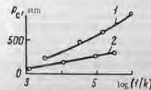
FIGURE 31. Critical pressure of collapse as a function of the logarithm of the reciprocal gas permeability of PETN ( d_{\text{charge}} = 10 mm):
