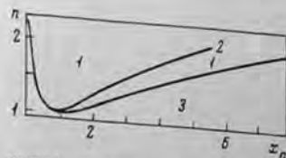
FIGURE 95. Instability region (1), wave numbers of the most dangerous perturbation (2), and region of absolute stability of burning (3).
