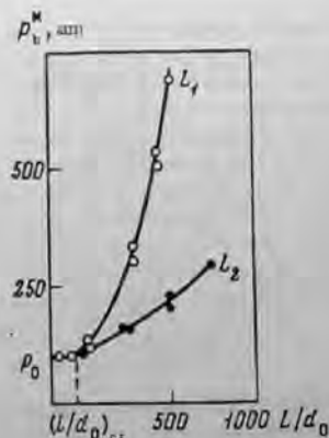
FIGURE 54. Excess pressure in fissures of various depths as a function of parameter (L/d_0) , L_1 > L_2 .
