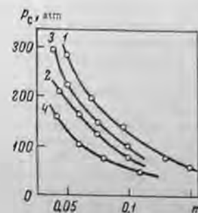
FIGURE 28. Critical pressure of collapse as a function of porosity for mixed explosives ( d_{\text{charge}} = 10 mm, r = 5-20 \mu ):
